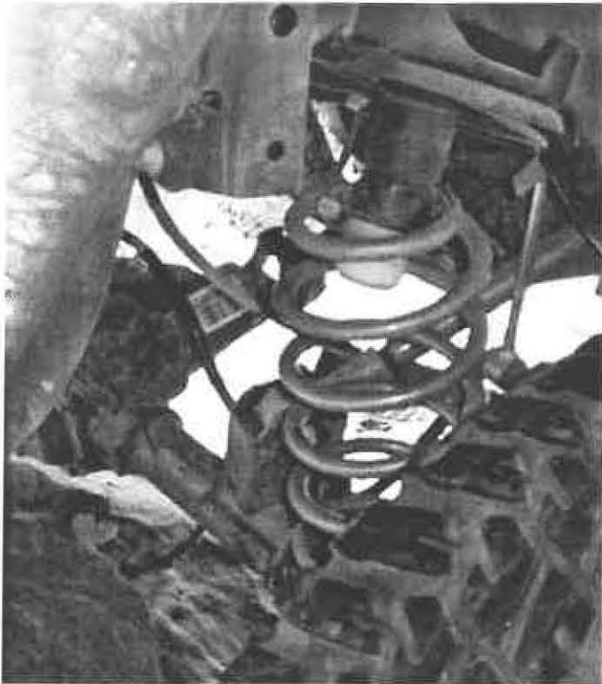
Mike's "3-shock" set-up Note the superior axle droop in Mike's "system"
