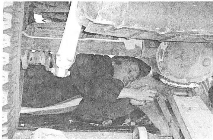
Kristy reinstalls her rear drive shaft after Jeff replaced a damaged U-Joint for her
