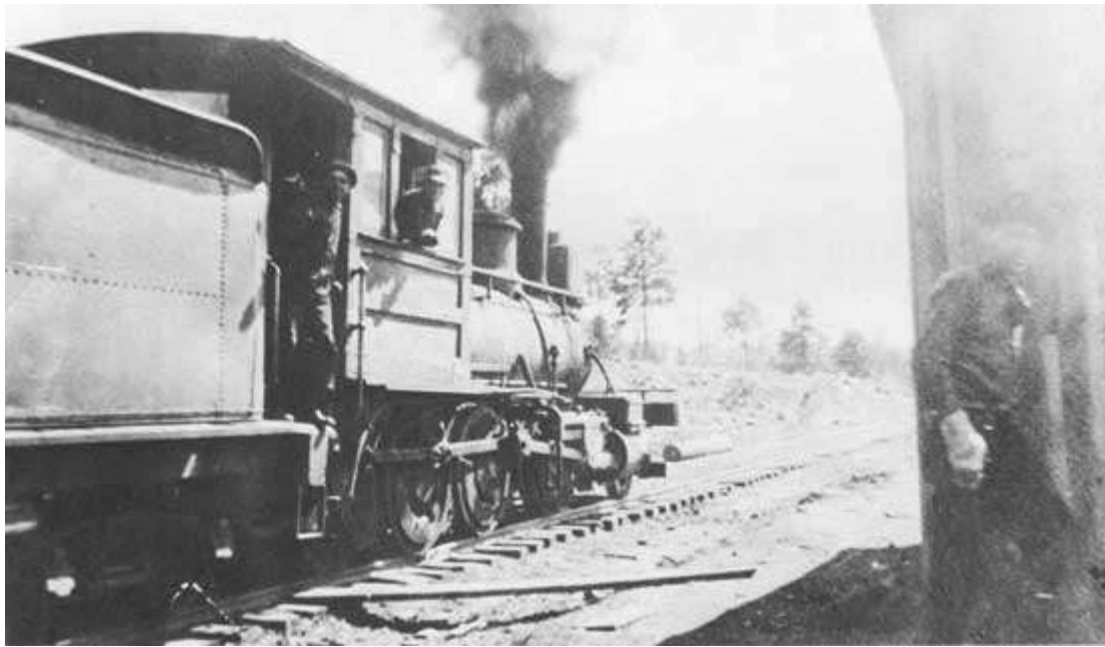
Figure 63. An old Santa Fe Railway freight locomotive on the Zuni Mountain Railway. This is probably Number 2303, an 1882 Hinkley leased or borrowed by the logging railroad circa 1906-1908. (John Bigley collection)
