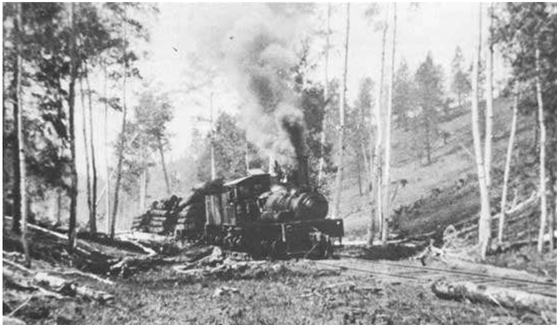
Figure 23. Shay locomotive Number 3 bringing in a train from the woods. ( John Bigley collection )
