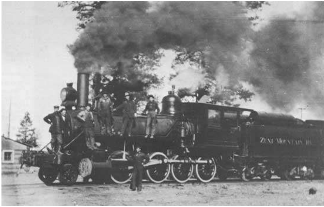
Figure 28. Old "mainline" locomotive Number 6 of the Zuni Mountain Railway. This ancient eight-driven freight locomotive was used to haul log trains from the woods camps to the connection with the Santa Fe Railway at Thoreau. ( Cibola National Forest collection )
