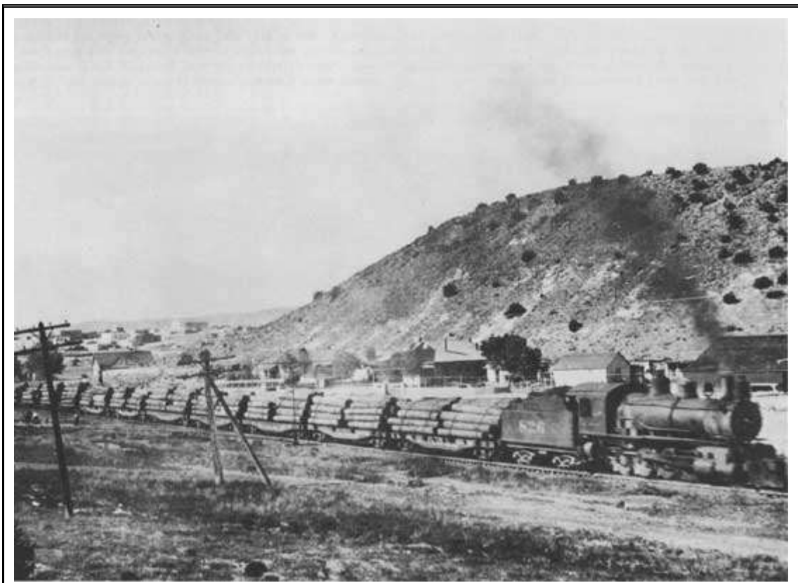
Figure 8. Santa Fe Railway locomotive Number 826 hauling a string of log cars through Laguna, New Mexico, in 1912. By this time, the train included a substantial number of Santa Fe Railway steel log cars, although several of the older Zuni Mountain Railway wooden log cars may be seen back in the train. ( John B. Moore, Jr., collection )
