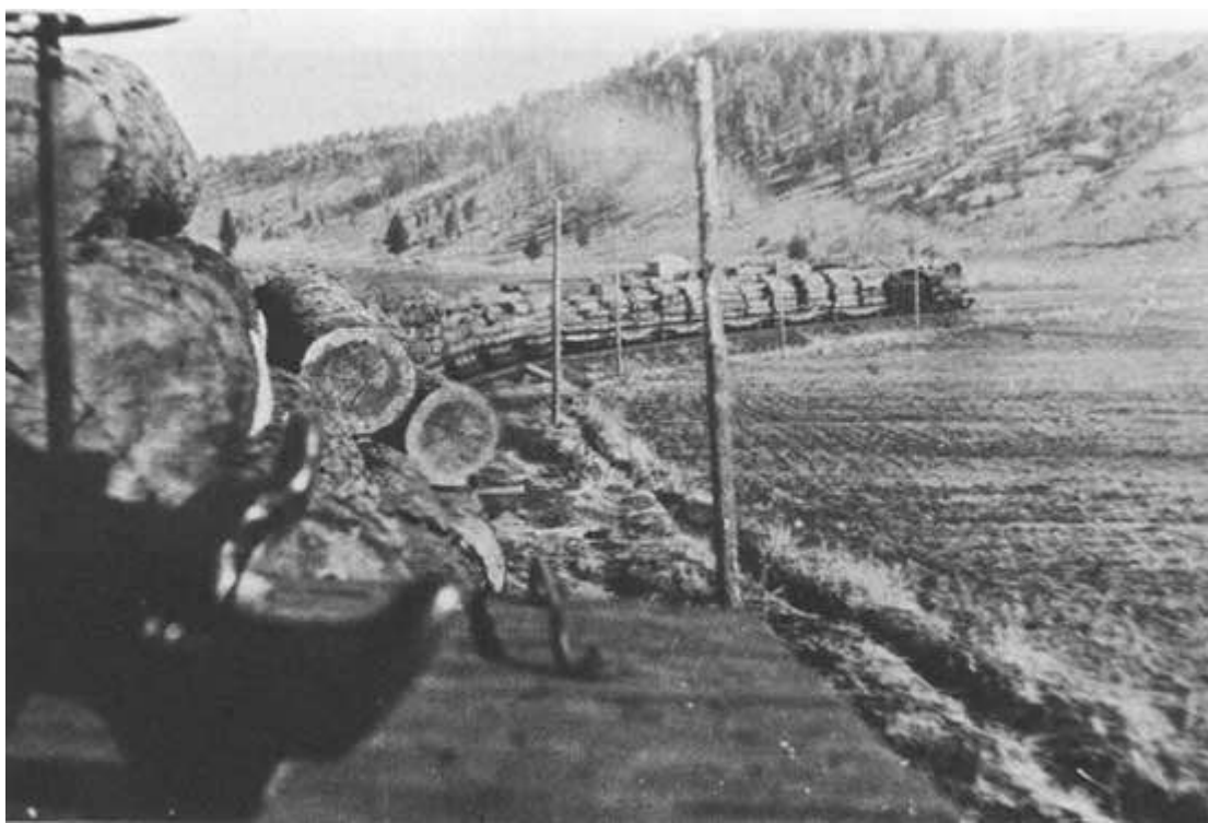
Figure 28. Old "mainline" locomotive Number 6 of the Zuni Mountain Railway. This ancient eight-driven freight locomotive was used to haul log trains from the woods camps to the connection with the Santa Fe Railway at Thoreau. ( Cibola National Forest collection )
