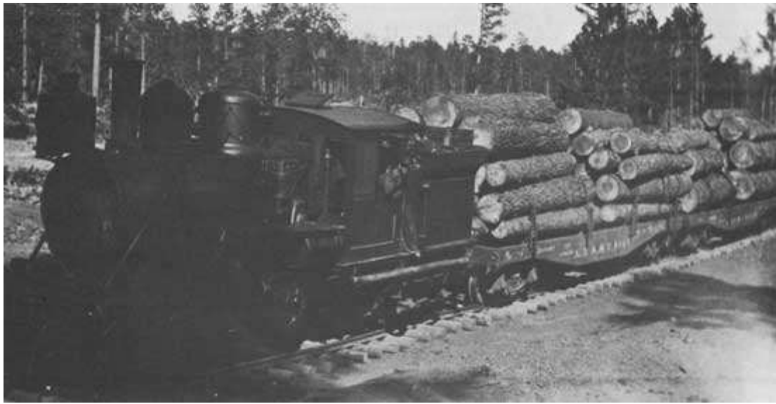
Figure 57. The Climax gear-drive locomotive, Zuni Mountain Railroad Number 8, heads for camp with loads of logs. ( Cibola National Forest collection )
