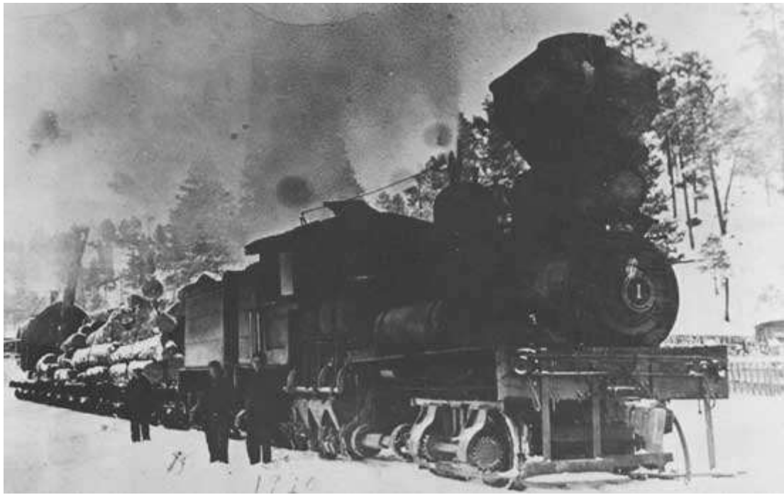
Figure 46. McGaffey Company Shay Number 1 was the woods locomotive. Jim Clark, the engineer, stood near the cab. By this time, the locomotive had lost its big wood pilot or "cowcatcher," and it had acquired a pair of rather spindly footboards. ( Susan Clark Kirk collection. Gallup Public Library Photo Archives #1322 )
