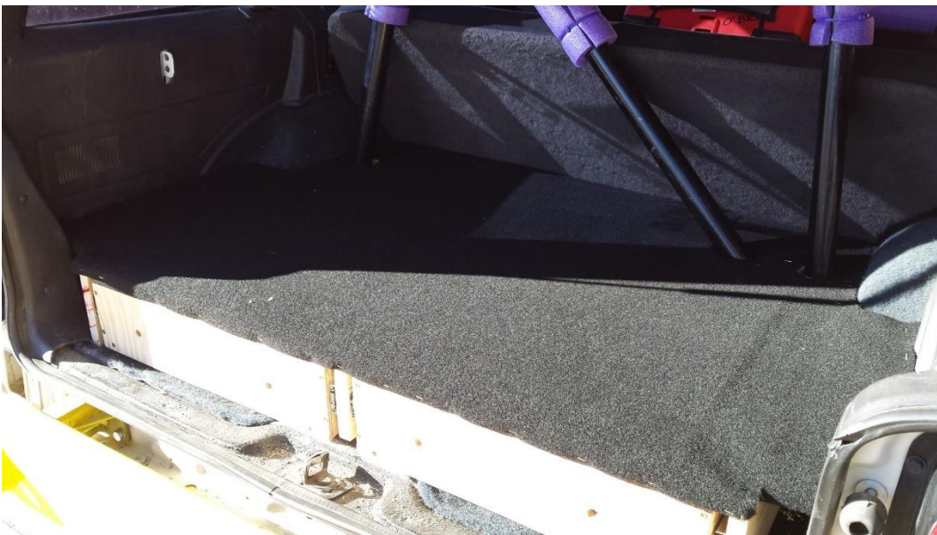
A roll of automotive carpet from Autozone covers the deck. I also added some sheeting between the rear seat and the C-pillar on the cage. The drawers don't extend that far, so I have more storage for things that don't get used that much (jack, chocks, etc), only accessible by pulling the seat back forward.
