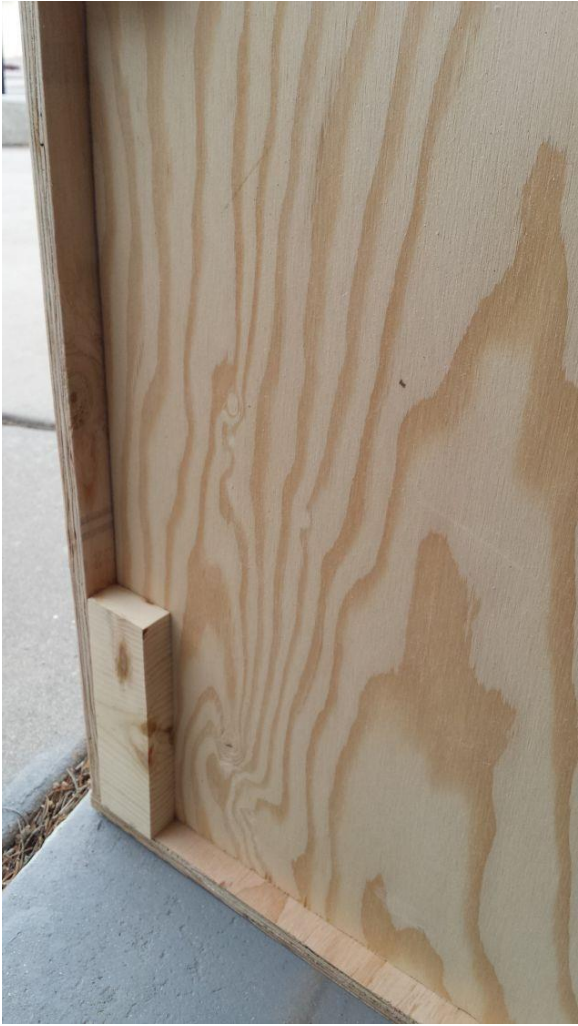
Bottom support for the drawers. Didn't want to try screwing into the sidewall of the plywood
