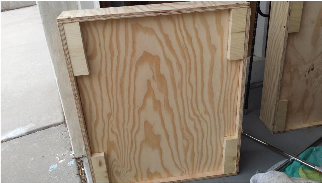
Bottom support for the drawers. Didn't want to try screwing into the sidewall of the plywood
