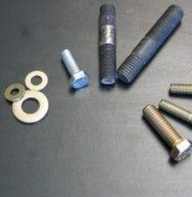
Figure 3 - Clockwise from left: Grade 8 flat washers, Grade 5 UNF bolt, UNF/UNF stud, UNC/UNF stud, Grade 8 bolts.
